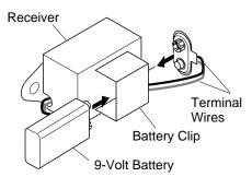
Figure 44 - Attaching Alkaline Battery to Receiver
